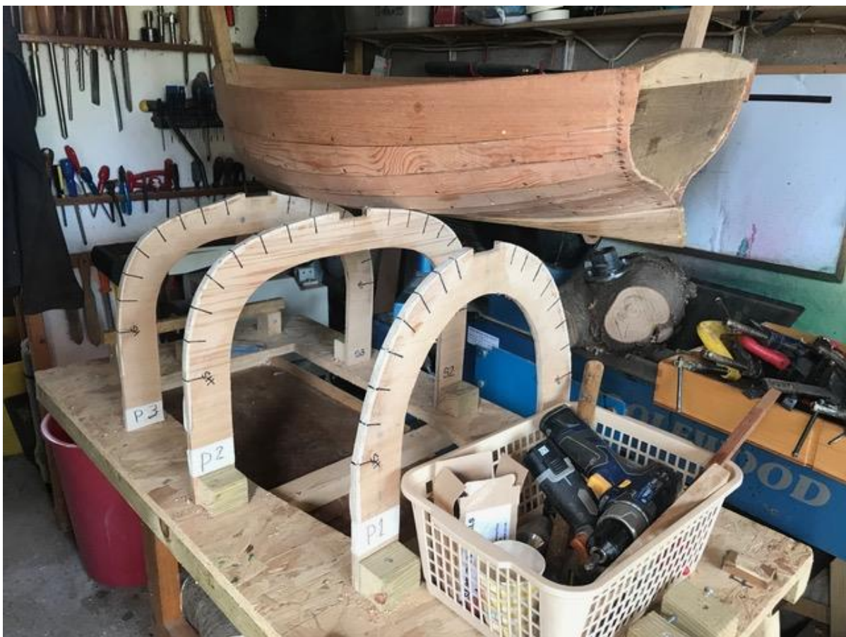
14ft Clinker dinghy just taken off the building moulds
